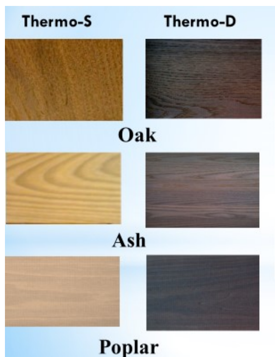
Fig. 4. The effect of Thermo wood- treatment on the colour of oak, ash and poplar. The treatment temperatures for Thermo-S - 185°C and Thermo-D - 215°C.
