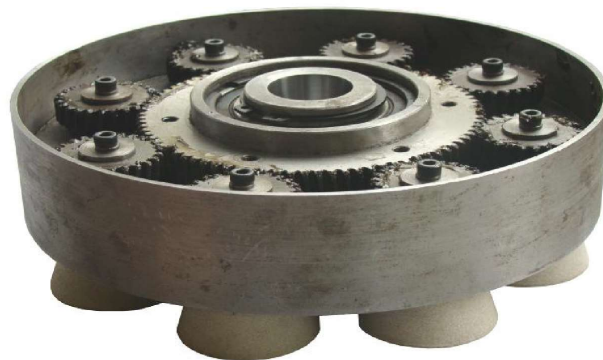
Fig.2. Orbital grinding tool for sharpening woodcutting planer knives: a – overall view; b – research prototype
